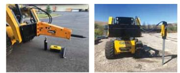
Photo at left shows Montana Breaker with chisel bit attached, and rounded bit and nitrogen kit. T-Rex post driver at right is shown equipped with a side extension.
