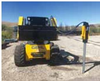
Photo at left shows Montana Breaker with chisel bit attached, and rounded bit and nitrogen kit. T-Rex post driver at right is shown equipped with a side extension.
