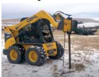
Post driver handles T-posts, and pipes up to 3 in. in diameter.
