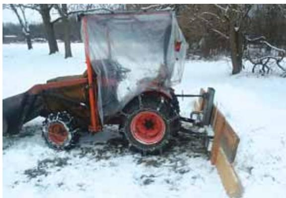
**"Poor man's" snowplow tractor is fitted with a home-built, 10-ft. wooden snow blade and a "shower curtain" cab.**
