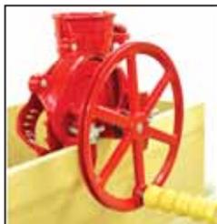
**Maximizer hand sheller's crank wheel comes with a pulley if you want to add a motor to power it.**
