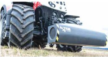
Top Soil Mapper identifies soil compaction depth on-the-go and tells you how deep to rip. It can be used with an automatic tillage control kit that installs on your cultivator or subsoiler.
