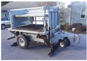
Hydraulic-driven front wheels on self-propelled hoof trimming table make it easy to back into tight spaces. A front jack stand raises wheels off the ground for hooking up unit's gooseneck hitch.
