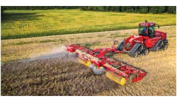
CrossCutter Disc works at a shallow depth, leaving crop residue at or near the surface. Discs are mounted on rubber-suspended arms to closely follow ground contour.
