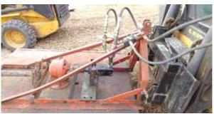
removed mower's pto shaft and installed a hydraulic motor to match the hydraulic output of his skid loader.
