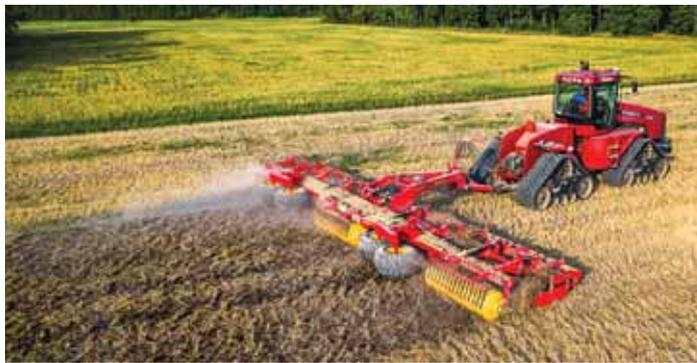
CrossCutter Disc works at a shallow depth, leaving crop residue at or near the surface. Discs are mounted on rubber-suspended arms to closely follow ground contour.
