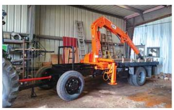
To convert boom truck to a trailer Cervany cut down the truck's frame, added a tongue on front, and reversed the front axle. He also extended linkage to truck's driveline so he could power the boom with a tractor pto.
