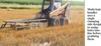
handler uses a single clamping side design to nudge bales into line before grabbing them.
