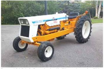
Repowered Cub Cadet Lo-Boy was lengthened by 22 in. to make room for a 500-hp., 7.3-liter Power Stroke diesel engine off a Ford F-350 pickup.
