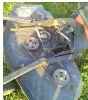
**Aaron Miller built a bigger 48-in. mower deck for his DR brush mower, using the pulleys and components from an old Deere mower.**
