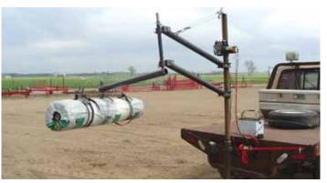
Pickup-mounted, winch-operated lifting device lets one man easily lift a roll of net
