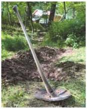
Swinging disk hoe was made by bolting a big coulter onto the end of a 45-in. hickory
