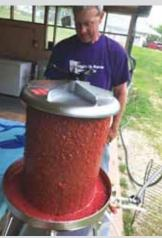
Jim Riddle uses his Hydropress to turn fresh fruit into juice. "It works faster than steaming and does a better job, and doesn't require any power other than a garden hose," he says.
