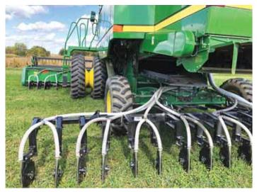
A 15-ft. toolbar with single disc coulters mounts on combine's rear axle, with 6-ft. toolbars mounted to each end of the 30-ft. sovbean header.
