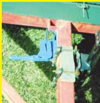
About 3 years ago I rebuilt my 5 by 8 utility trailer. I used an axle from a 1970 military jeep trailer because it had a parking brake (lever shown in blue in the picture). It's great because I was tired of having to put a 2 by 4 block behind the wheels of my old trailer whenever I parked on an incline. **(Wayne A. Beggs, Lincolnton, Ga.)**
