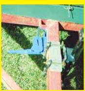
About 3 years ago I rebuilt my 5 by 8 utility trailer. I used an axle from a 1970 military jeep trailer because it had a parking brake (lever shown in blue in the picture). It's great because I was tired of having to put a 2 by 4 block behind the wheels of my old trailer whenever I parked on an incline. (Wayne A. Beggs, LincoInton, Ga.)
