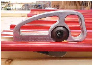
Handheld "slitter" uses a pair of overlapping 2-in. dia. cutter wheels to cut through metal up to 24-ga. thick.
