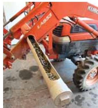
Foley stores chains and tools in a 4-in. dia. pvc tube on his Kubota loader tractor, cutting a wide slot along the top and threading a pvc cap onto the tube.
