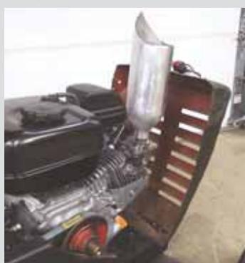
**Lee Shepherd, Wabash, Ind.:** Lee runs a small engine repair shop for lawn and garden tractors. He recently made a custom exhaust "tip" out of an old fire extinguisher that he had laying around. It sticks off the front of one of his tractors and is a real eye-catcher.
