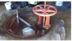
Turning a rotary wheel on gate valve causes a threaded shaft to push a pad against tire bead and break bead off wheel rim.
