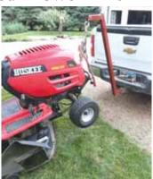
To lift his riding mower, Meiners jacks up a come-along that has cable attached to mower's front bumper.
