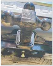
Larry Wood, Waldo, Ohio: "Tired of your trailer making noise when you travel down the road? I have a Ford F-350 with a 2 ½-in. receiver hitch so I use a sleeve adaptor so our 2-in. ball hitch will work properly. But each time I pulled the 2-in. hitch out to change the ball size, the sleeve would move and pinhole would be misaligned.
