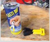
James Minix, Morrison, Tenn.: "I was having trouble keeping plastic electric fence insulators from breaking prematurely on chain link fence due to sunlight causing them to get brittle and weak. So I got the idea to protect them by coating the end of the connector that attaches to the fence with Plasti Dip that people normally use to coat handles on shop tools. It seems to work well, extending the life of the insulators by protecting the plastic from the sun."
