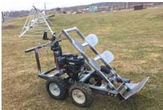
Cradle on motorized carrier tips back, allowing Sager to pick up a 4 to 5-ft. section of log or even a big stump - and carry it away.
