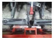
Carrier hooks up to quick-tach mounting brackets on 3-pt. hitch.
