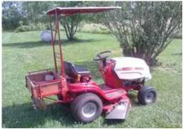
Removable canopy and bed attach to riding mower without any welding.
