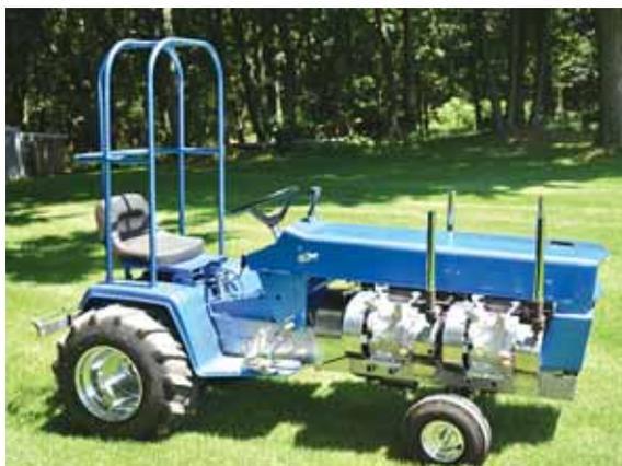
Garden tractor puller is powered by four 8 hp. Harbor Freight Predator V-twin engines.
