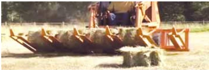
**Bale Sweep can be used with a skid loader or front-end loader. "The forks follow the contour of the ground without digging in," says inventor George Krizenawski.**
