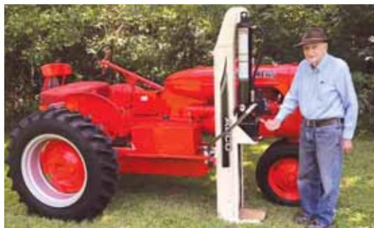
**Worth Harman mounted a SpeeCo SplitMaster wood splitter alongside his Allis Chalmers C tractor. It's powered by a pump that runs off the pto.**
