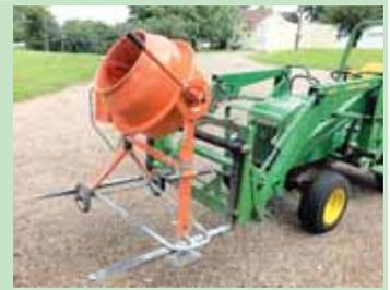
**Mark Rinke mounted a cement mixer on his front-end loader, and built a jig for the tractor's 3-pt. hitch so he could move a 25-ft. storage container into place.**
