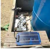
Sprayer pump is powered by a 12-volt battery that is recharged by a solar panel.
