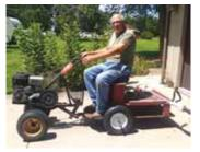
Sieber replaced walk-behind tiller's tines with wheels, and attached the power unit
