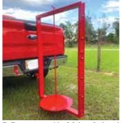
Ez Fenzer comes with a 2-ft. long, L-shaped "drop hitch" bracket that attaches to fencer and fits into pickup's receiver hitch.
