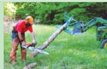
Log picker attaches to loader forks and holds log about waist high, making it easy to cut off pieces.
