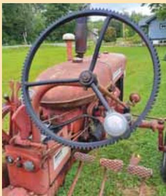
Anderson welded the ring gear to the tractor’s original steering wheel spokes, keeping the steering knob.
