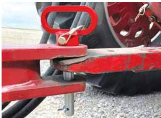
Quick-Pin comes with a top sleeve held by a locking pin, and a shaft with a hole near the top. Removing the locking pin leaves just the shaft in the hitch, and the tractor operator releases pressure on the shaft, it falls through.
