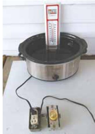
Crockpot plugs into a 110-volt wall outlet that's wired in series to a dimmer switch, which lets Forsy lower crockpot temperature to just above freezing.
