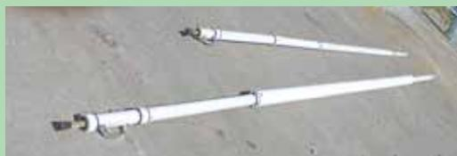
One end of each tube attaches to board on top of auger, and the other end lodges against bin wall.
