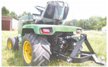
Bill Ruegg says his 3-pt. hitches for Deere lawn tractors work great for plowing, disking, blading and so forth. Photo shows hitch kit on a Deere 318.
