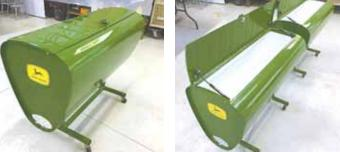
Jim Heitkamp serves up beverages out of a pair of converted Deere fertilizer hoppers. Stands with wheels were welded to the bottom of hoppers, which are lined with styrofoam.
