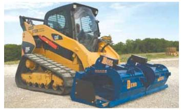
Demo-Dozer skid loader attachment can be used as a dozer, clam bucket, material bucket, log handler, 4-in-1 bucket, receiver hitch, or demolition grapple.
