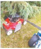
Deflector allows add-on mower to go all the way under lower boughs of evergreens without catching.
