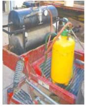
Nahrwold made a pressurized sprayer for his riding mower by plumbing together 2 air tanks from truck brakes, then running an air hose from them to a 3-gal. sprayer.
