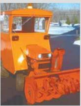
Home-built cab is equipped with a wiper, defroster, 15,000 btu heater, mirrors, flasher, and extra lights. Johnson rebuilt the snowblower.
