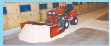
The 5-ft. wide Spread-Rite spreads poultry bedding quickly and evenly. It's designed for use with Ventrac and Steiner tractors.
