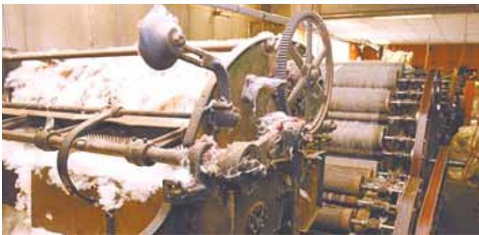
Photo shows wool fiber being loaded into carding machine at Green Mountain Spinnery.
