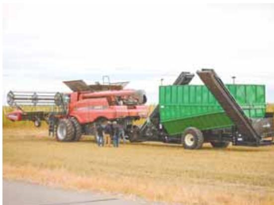
The Grass Hopper, a large wheeled tank, can be pulled behind a combine to collect plant residue. A conveyor delivers material into cart, which unloads it into a truck or trailer at edge of field.
