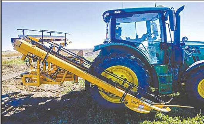
Bish's tractor-mounted, hydraulic-powered hemp harvester cuts the stalk at ground level and conveys it to a wagon or trailer pulled alongside harvester.
