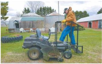
Bob Manzke demonstrates how he uses add-on steps and handrails, built by son Russ, to climb onto mower deck.
