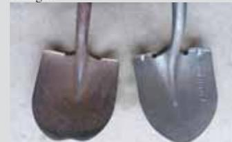
**Dave Meiners, Edgerton, Minn.:** "I used a torch to cut a big notch in the pointed end of my shovel and then used an angle grinder to sharpen it. Makes the tough work of digging a little easier because the shovel can penetrate hard soil with less energy and more balance."
