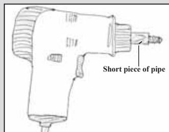
**Raymond Rodriguez, Waxahachie, Texas:** "To avoid hitting electrical wires when drilling into walls, I just slip a small piece of pipe over the drill bit to keep the bit from going in too deep. Just make the
