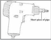
Raymond Rodriguez, Waxahachie, Texas: "To avoid hitting electrical wires when drilling into walls, I just slip a small piece of pipe over the drill bit to keep the bit from going in too deep. Just make the
