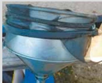
**Gary Swensen, Yankton, S. Dak.:** "The little screen in the bottom of a funnel came loose and ended up in the bottom of my fuel tank. Instead of throwing the funnel away, I made a big screen from some window screen and a tarp strap. It goes over the whole top of the funnel. It won't win a beauty contest but it keeps my fuel clean and it won't fall out of the funnel."
