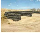
Compacted rubber bales measure 5 by 5 by 2 1/2 ft. and weigh one ton. They work great for everything from windbreaks and snow fences to storage bins.
