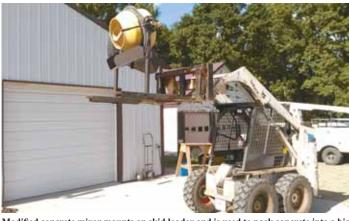
Modified concrete mixer mounts on skid loader and is used to pack concrete into a big culvert used as a roller. Chutes on both sides allow concrete to be dumped in either direction.
