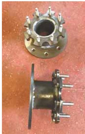
Adapters bolt onto standard skid loader hubs, allowing the use of low-cost truck tires. They're larger than skid loader tires so operators can drive 30 percent faster.
