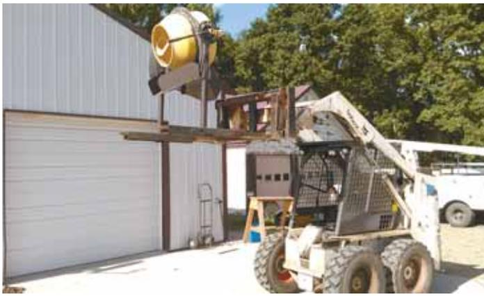
Modified concrete mixer mounts on skid loader and is used to pack concrete into a big culvert used as a roller. Chutes on both sides allow concrete to be dumped in either direction.
