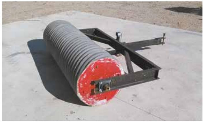
McLaen used 6-in. wide, 1/4-in. channel iron to build a frame for the 6-ft. long, 24-in. dia. roller.
