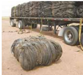
Compacted rubber bales measure 5 by 5 by 2 1/2 ft. and weigh one ton. They work great for everything from windbreaks and snow fences to storage bins.
