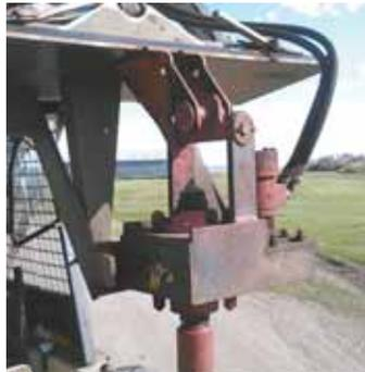
Auger head can still pivot forward and back and side-to-side.
