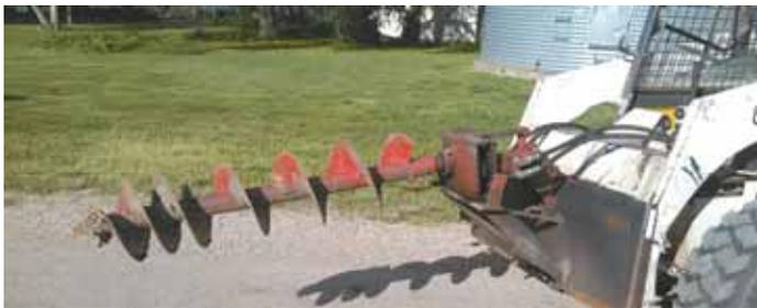
McLaen replaced the clamp that bolted to his loader bucket with a quick-tach plate that attaches to his skid loader. Auger rests in a saddle when in transport mode.
