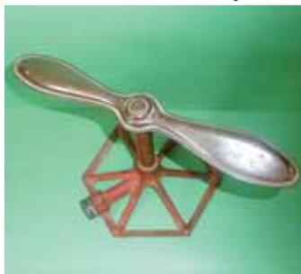
L.R. Nelson Co. sprinkler from the 1950's has a 12-in. propeller blade on a 9-in. sprinkler head. Monkey sprinkler holds its "tail" and spins as it sprays water.
