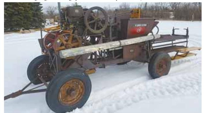
Workers rode on either side of the bale chamber to tie off the bales with wire.
