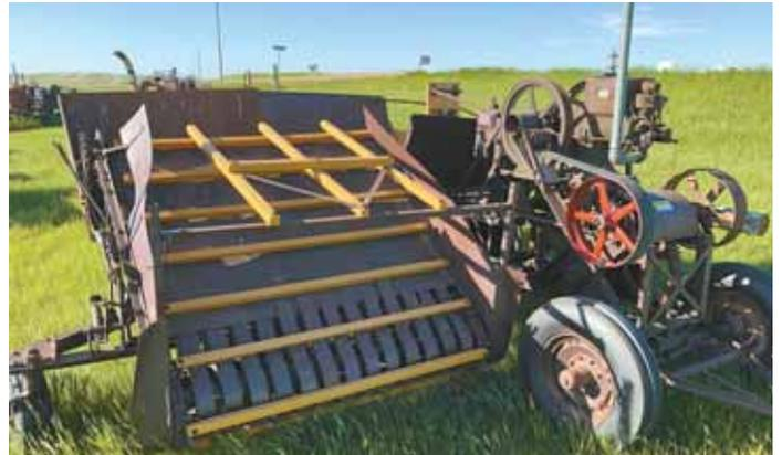
IHC no. 14 baler was built in 1940. It required a driver and a worker with a pitchfork to move the picked-up hay into the bale chamber.
