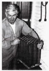
These 33 pipes mount between the stove and flue and are enclosed in a metal chamber. Smoke and ash pass up through them while room air is heated as it blows across them.
