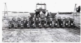
In only about 15 min. row units can be added or removed in switching the Nodet from one crop to another.
