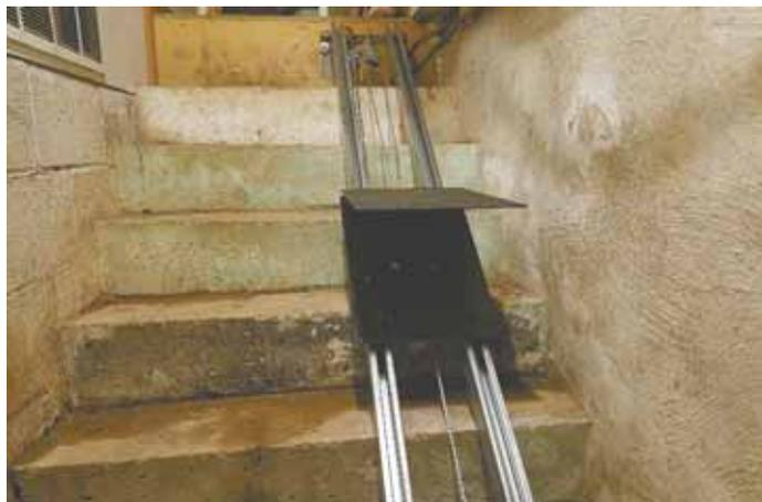
**Gary Nye used tracks from an old sliding barn door to make this simple lift. Metal platform rides on wheels inside tracks.**
