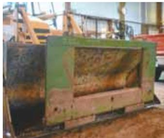
Mills mounts part of a feederhouse off a junked Deere combine on his loader tractor to lift his Deere 920 combine head off its transport cart (above). Loader is then tilted up until skids are nearly vertical and at a convenient working height.
