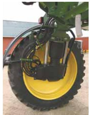
“On a Deere sprayer with 46-in. wheel rims, our lift kit will provide up to 71 in. of clearance,” says Simon. Large strut rods guide the lift system as it moves up and down.
