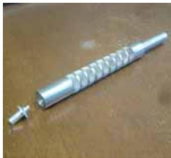
A “driving pin” extends out one end of tool. Operator pushes rivet through poly skid and backing plate, and then uses a hammer to hit the driving pin.
