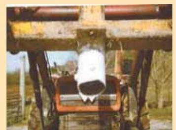
**Lawrence uses short piece of pipe welded to bottom of bale spear to push metal fence posts into the ground.**
