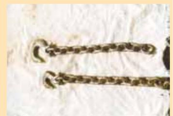
**Lawrence converted a grab hook chain to a slip hook chain by cutting off the top 1 ft. of a slip hook chain and slipping the bottom link onto the grab hook.**
