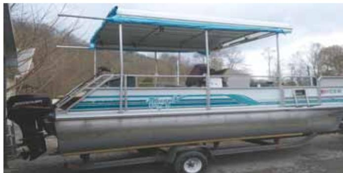
Plunkett replaced the small vinyl roof on his pontoon boat with a bigger one made from sheet metal siding.
