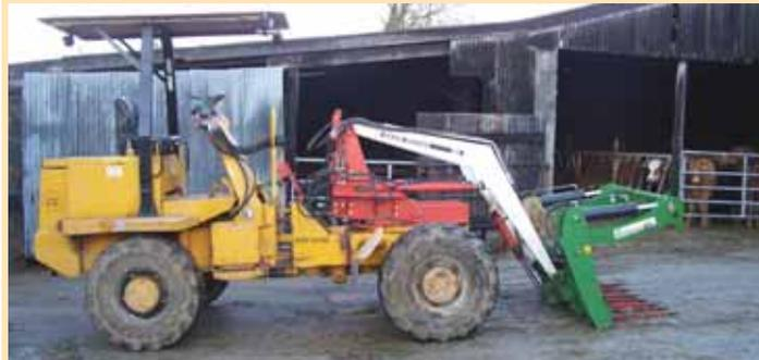
Loader attaches to a frame that pivots 180 degrees and is fitted with lift cylinders.
