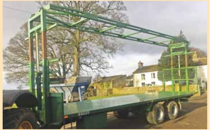
Hydraulically-controlled cage on trailer clamps down on top of bales once they're loaded, eliminating the need to strap them down.
